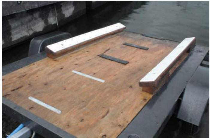
*Photographs by the author - The HDPE strips and StarBoard-covered bunks made moving the boat off and back on the trailer much easier than the bare plywood deck and carpet-padded bunks did.*
