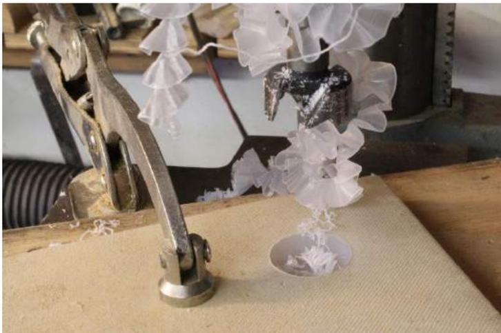
High-density polyethylene is as easy to work as softwood. This 1" Forstner bit cut right through the 1/2"-thick panel.
